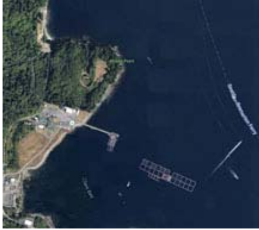
Figure 7. Left overview of pier and research net-pens at NOAA's Manchester laboratory. Right, detail of pens. Pens in orange border do not touch the bottom at low tide. Each pen is: 16'x 16' x 12' WxLxD. Pens in yellow border touch the bottom at low tide.
